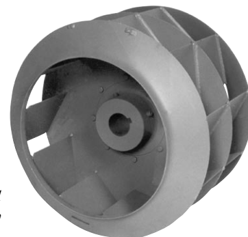
DWDI airfoil wheel with die-formed hollow airfoil blades continuously welded to the rim and backplate.
