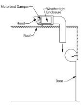
The door air heater is very effective when mounted outside as illustrated at right. Include weathertight enclosure option. Rain shield is to be furnished by the installer.
