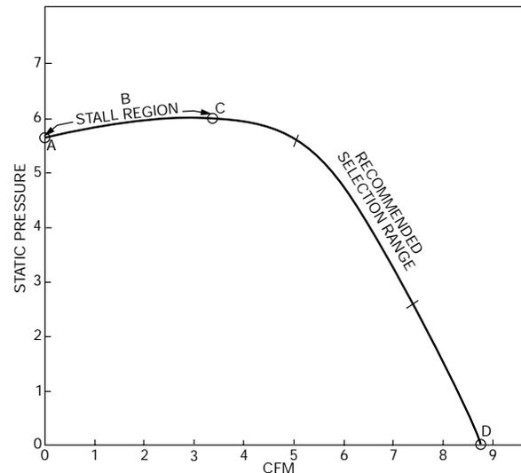
curve for a backward inclined centrifugal fan. This curve shape is also representative of radial blade centrifugal fans.
