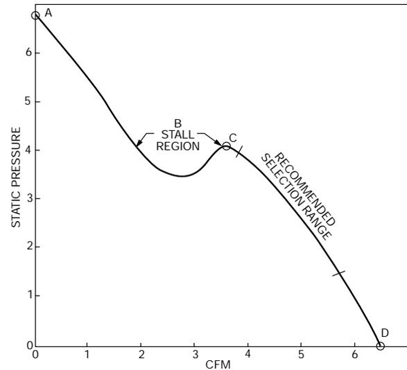
Figure 2. Static Pressure Curve, Backward Inclined Centrifugal
