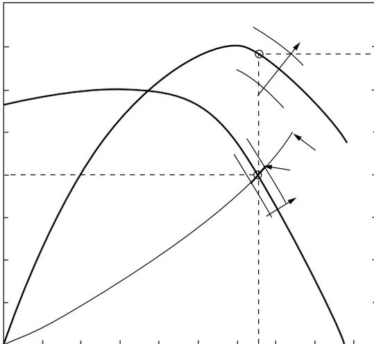
These speed changes represent an example of fan control that can be accomplished through drive changes or a variable speed motor.
