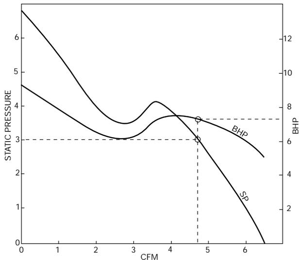
By adding the BHP curve to the static pressure curve from Figure 3 we complete the fan performance curve. To determine BHP simply extend vertically the CFM point established in Figure 3 until it intersects the BHP curve. Draw a horizontal line from this point of intersection to the right to the BHP scale to establish a BHP of 7.27 units, which corresponds to the previously established performance of 4.71 CFM units at 3.0 SP units.
