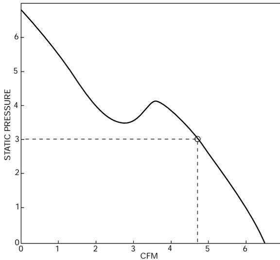
Simply locate some unit of pressure on the left hand SP scale and project a horizontal line to the point of intersection on the static pressure curve. From the point of intersection project a vertical line to the bottom CFM scale to establish the corresponding airflow at that particular speed. In this example a static pressure of three units results in a CFM of 4.71 units.
