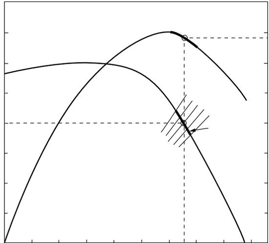
Combining the fan control curve (Figure 7) with the system controlled curve (Figure 8) results in a fan/system controlled curve having an "operating region" as shown in Figure 9.
