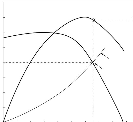
The system line is simply a parabolic curve made up of all possible SP and CFM combinations within a given system and is determined from the fan law that SP varies as RPM<sup>2</sup>. Another fan law states that CFM varies as the RPM. Therefore, we can also say that SP varies as CFM<sup>2</sup>. **Note:** Some systems have modulating dampers which will not follow this parabolic curve.
