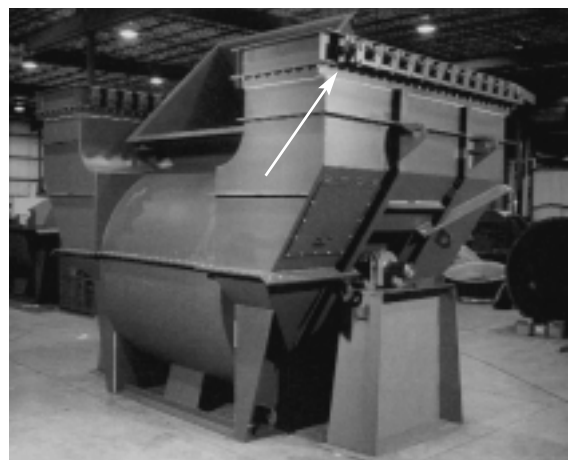
Figure 8. Inlet Box Damper
