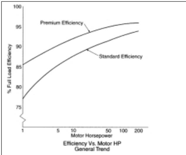
Converting electrical energy to mechanical energy is never perfect. It does become easier to approach 100% perfection with large motors than with small. The efficiency of standard industrial three phase motors usually runs from a level of approximately 75% at 1 HP to 94% at 200 HP.
