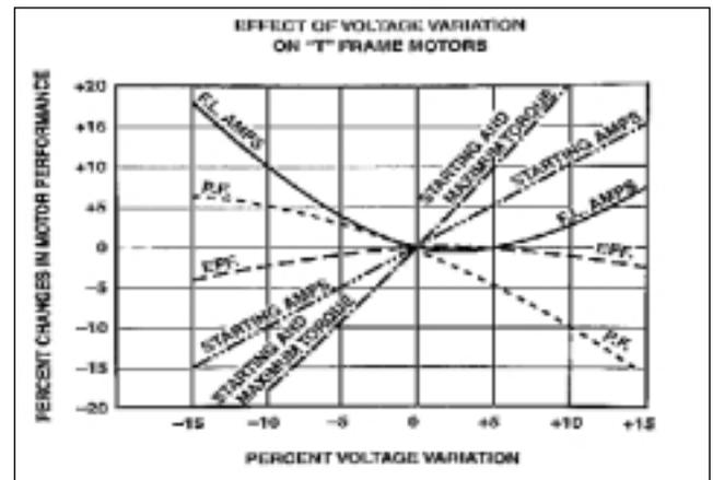
For example, the lowest point on the full load amp line does not always occur at 2% above rated voltage. On some motors, it might occur at a point below rated voltage. Also, the rise in full load amps above rated voltage tends to be steeper for some motor designs than others.
